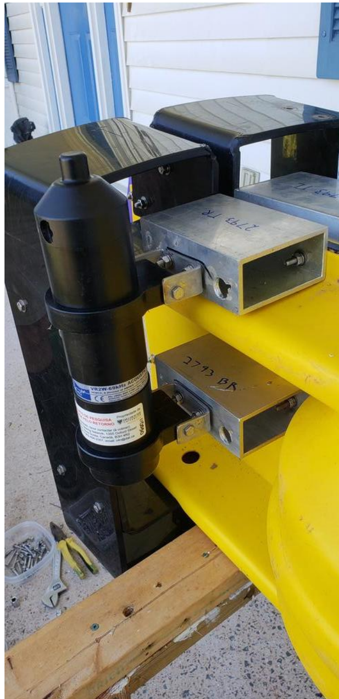
Figure 3: VR2W receiver mount
