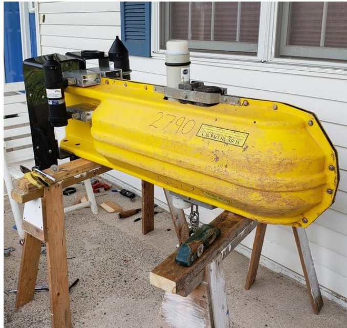
Figure 1: Picture of the SUB buoy with: (1) C-POD mounted in the middle, HR2 receiver mounted in front of the right side of the tail, and VR2W receiver mounted in front of the left side of the tail.
