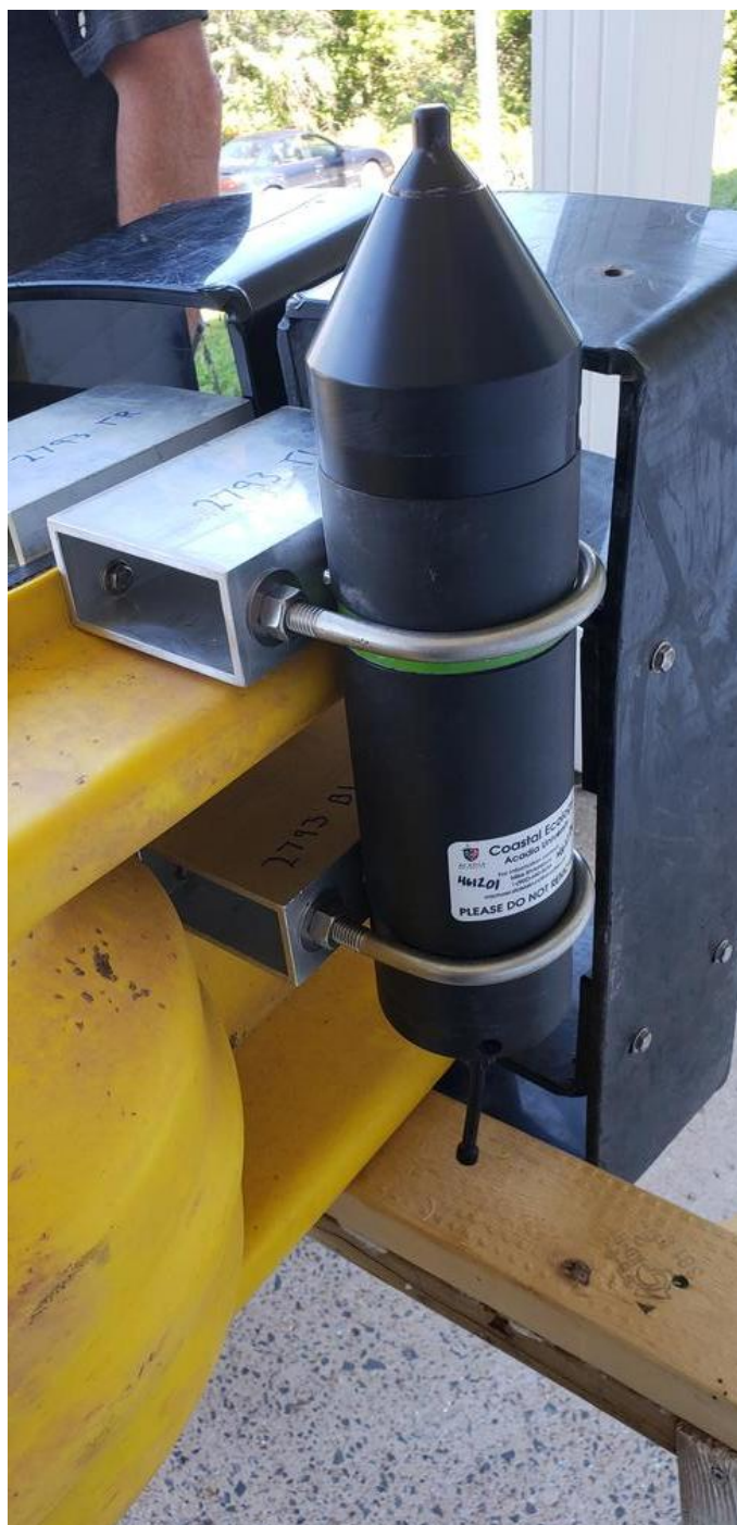
Figure 2: HR2 receiver mount
