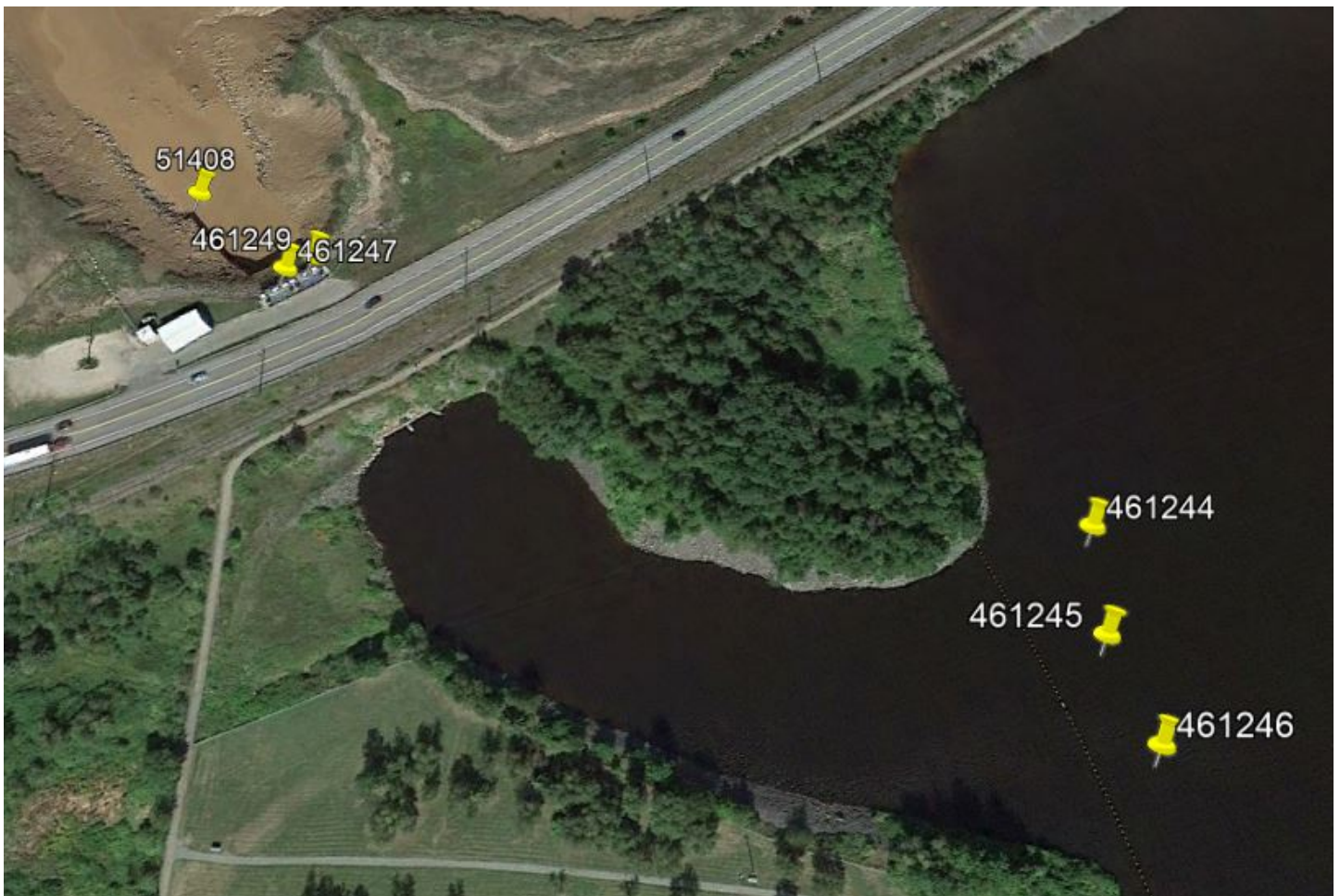
Figure 5: Equipment deployed, showing the test tag on the ocean side and the HR2 receivers on the impoundment side of the causeway. Straight line distance from the impoundment receivers to the gate receivers is about 230 m.
