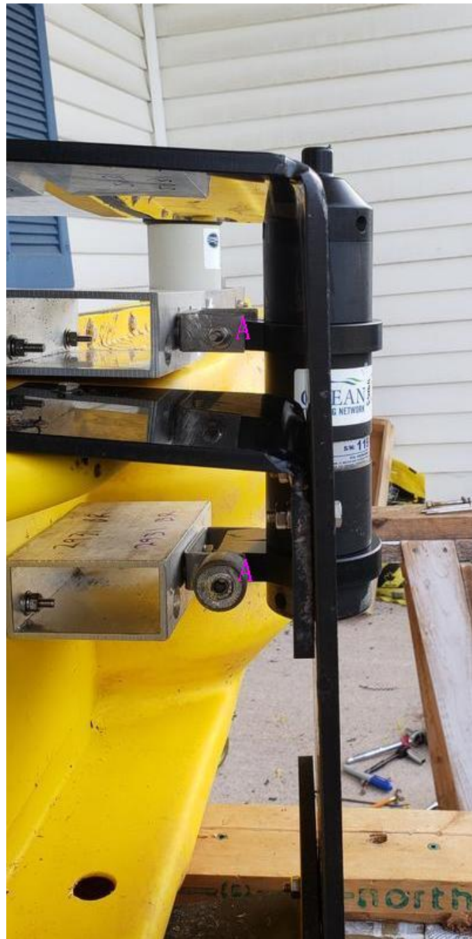
Figure 4: Anode attachment points on the protruding end of the retaining bolt for mounting the VR2W receiver.
